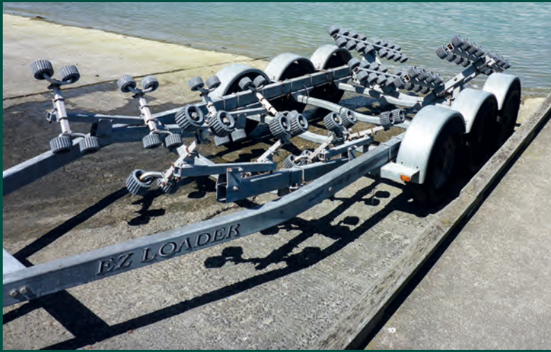
A whole lot of rollers on the E Z Loader trailer – nearly 100 – make for easy launching and retrieving.
