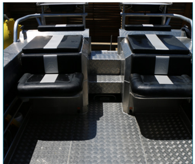
▲ Access to the full width-boarding platform is via a built in step as part of the engines cover.
