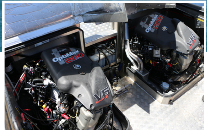
▲ The hearts of the operation, the two Mercury 200hp Optimax Sport Jets.
