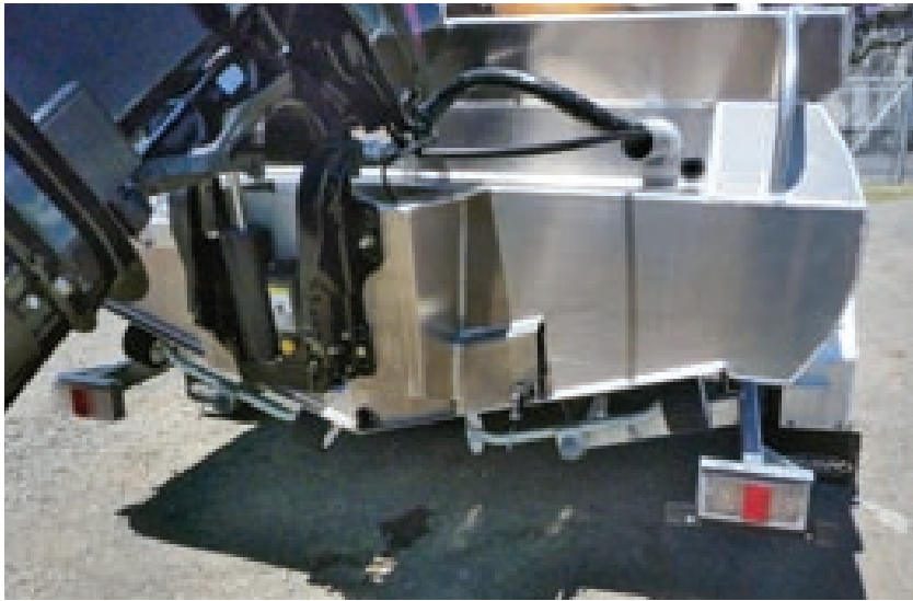
A separate transducer mounting plate removes the need to drill holes in the transom.
