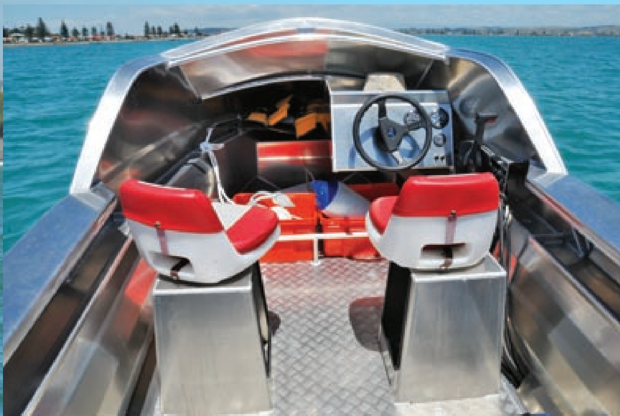
Rails constrain gear stored in bins in the bow.
