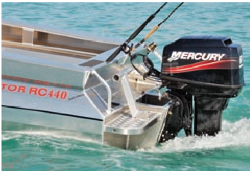
Boarding ladder and fold-down ladder are diver-friendly.
