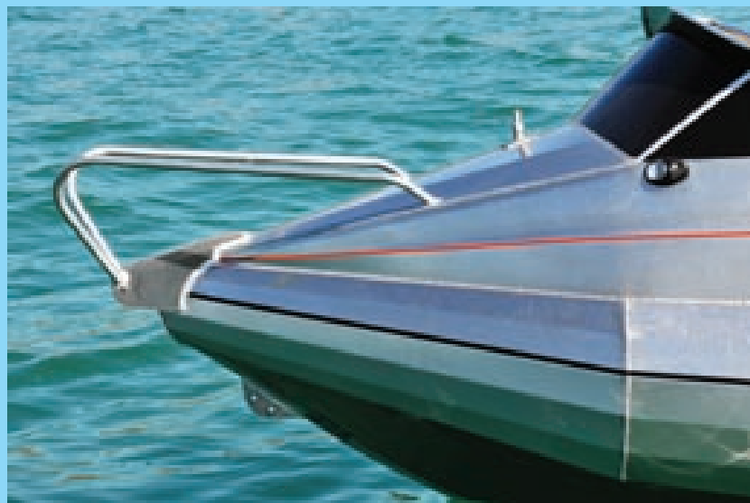
The bow rails constrain the anchor warp in the fairlead and it is easy to flip it in from the helm position.
